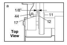
Screw (44) and move the Reed Switch slightly. Retighten the Screw. Re-attach the hood and run the treadmill for a few minutes to check for a correct speed reading.
